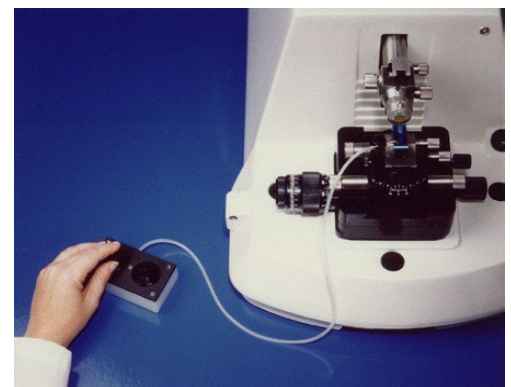
WATER TROUGH FILLER (PERISTALTIC WATER PUMP)
