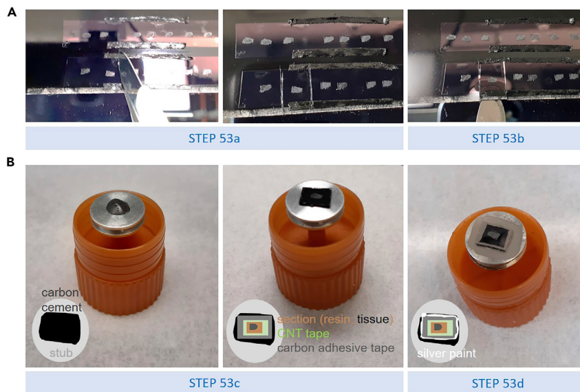
Figure 8. Remounting a section of interest onto a FIB stub
