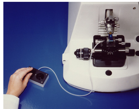
WATER TROUGH FILLER (PERISTALTIC WATER PUMP)
