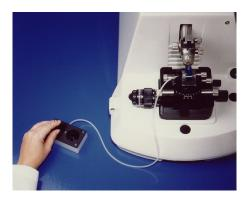
WATER TROUGH FILLER (PERISTALTIC WATER PUMP)
