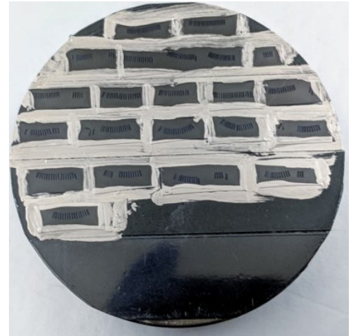
Figure 8. Strips of tape containing section ribbons is then mounted onto imaging substrates (e.g. 50mm SEM stubs).
