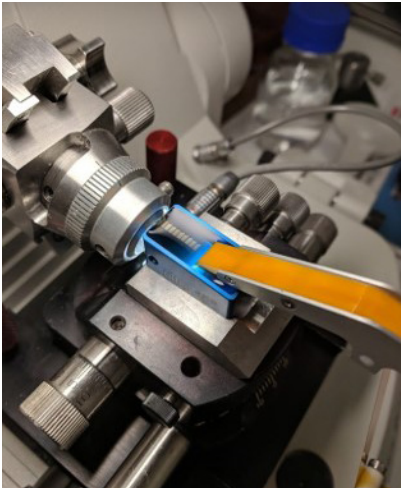
Figure 6. Ribbon of sections after being decompressed and manipulated in the trough toward the tape edge in preparation for collection.
